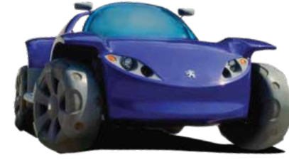
The PEUGEOT TOUAREG PEUGEOT's first-ever hybrid 4x4, with a single-cylinder engine, which acted as a generator.
